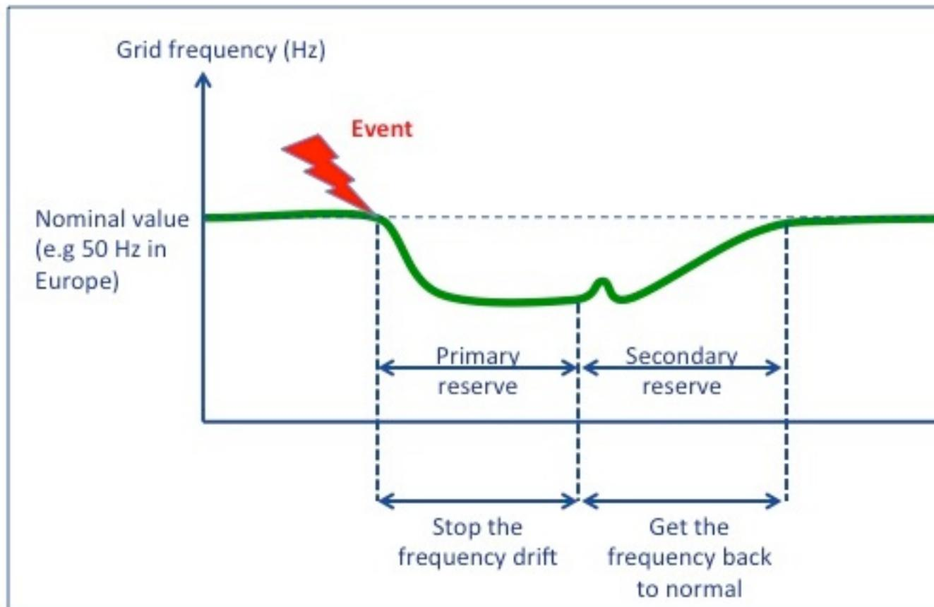
*Figure 1: frequency regulation with primary and secondary reserves*
