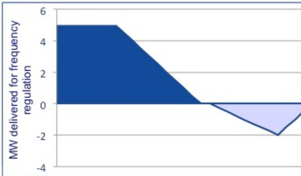
Figure 4: energy supplied by a slow asset for frequency regulation
