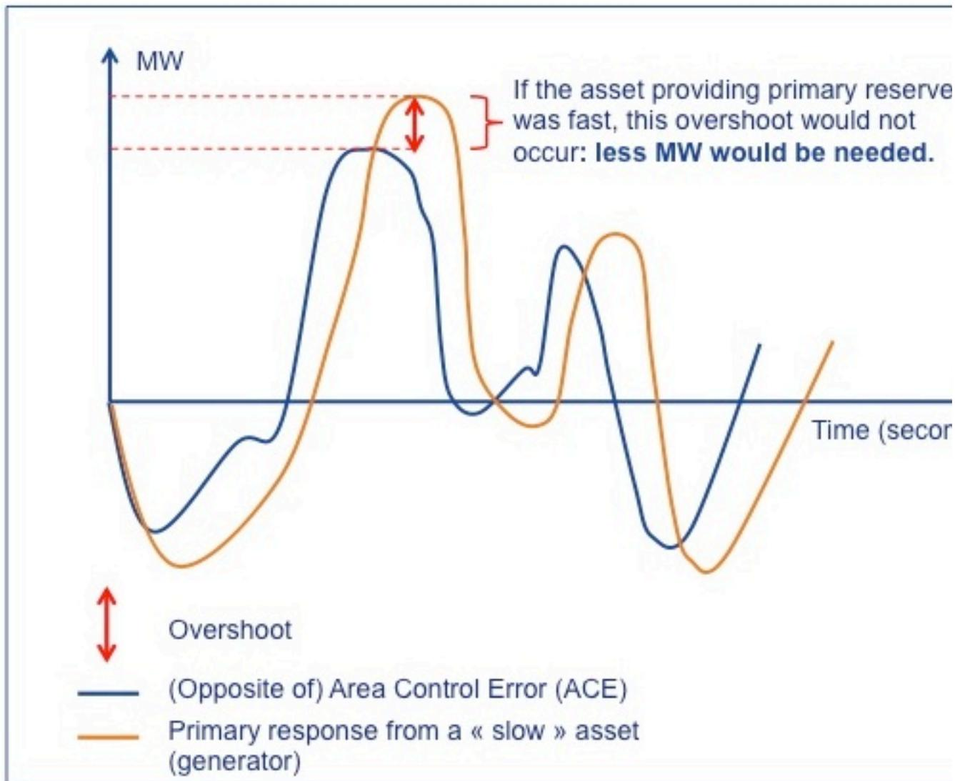
Figure 6: poor quality of response to frequency correction signal by a slow asset
