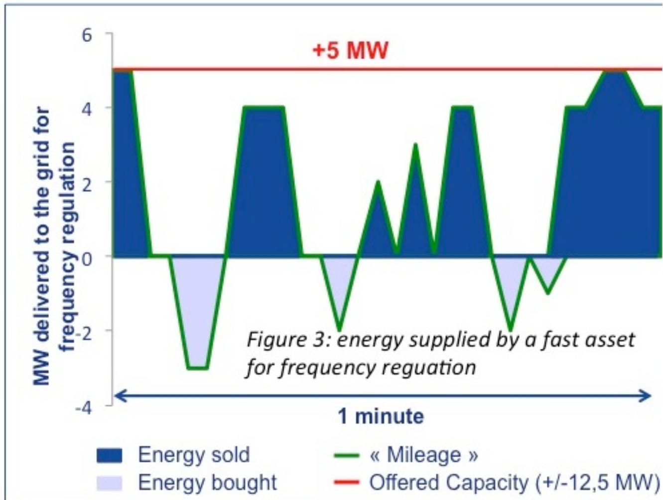
*Figure 5: principle of mileage measurement*
