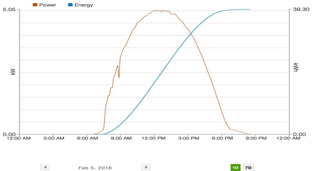
What is absolutely clear from the above output, is that I am producing worthwhile power during the actual peak demand for Victoria, and for some hours after the actual peak shown on the load curve. Using data from my smart meter I can add the actual demand I make on the grid, as below:
