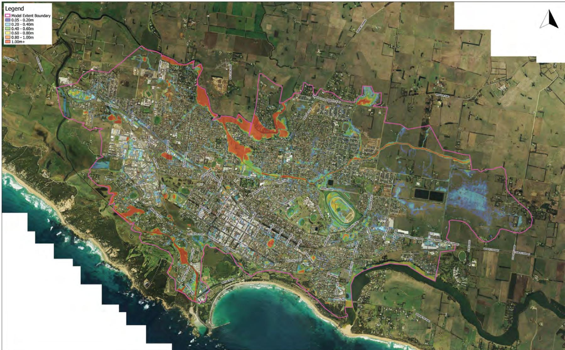
Figure 20. 1% AEP flood extents/depths under climate change scenario (Engeny, 2016)
