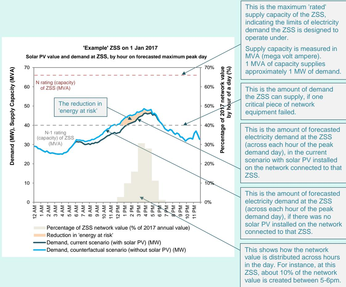
Distributed generation will provide value to the network when it reduces the amount of 'energy at risk'.<sup>46</sup> In the example above, distributed generation is providing value between the hours of 12pm and 6pm, because it is reducing the amount of energy that may be 'at risk' if the most critical piece of network equipment fails at that ZSS.
