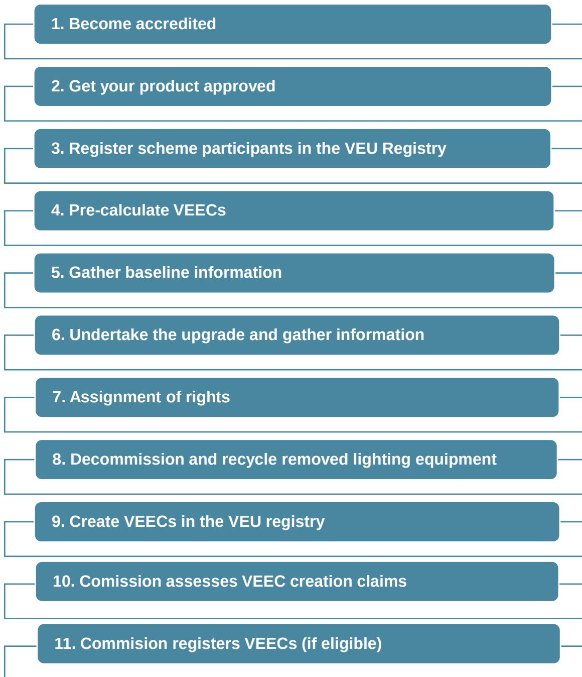
Figure 3: Process for undertaking building based lighting upgrades
