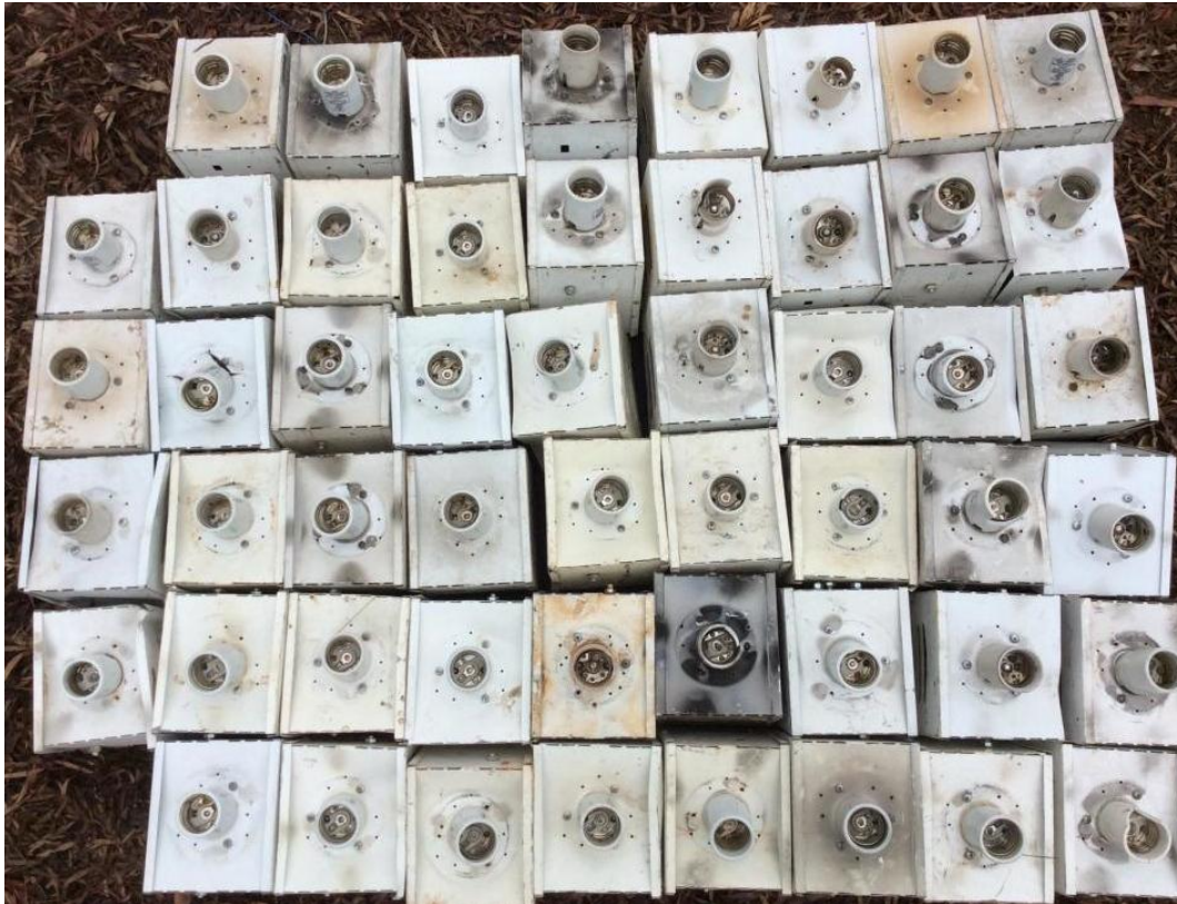
Figure 7: Example of a geo-tagged photograph of the removed ballast boxes of high-bay lamps lined up in a row with the lamp holders facing up and in focus.
