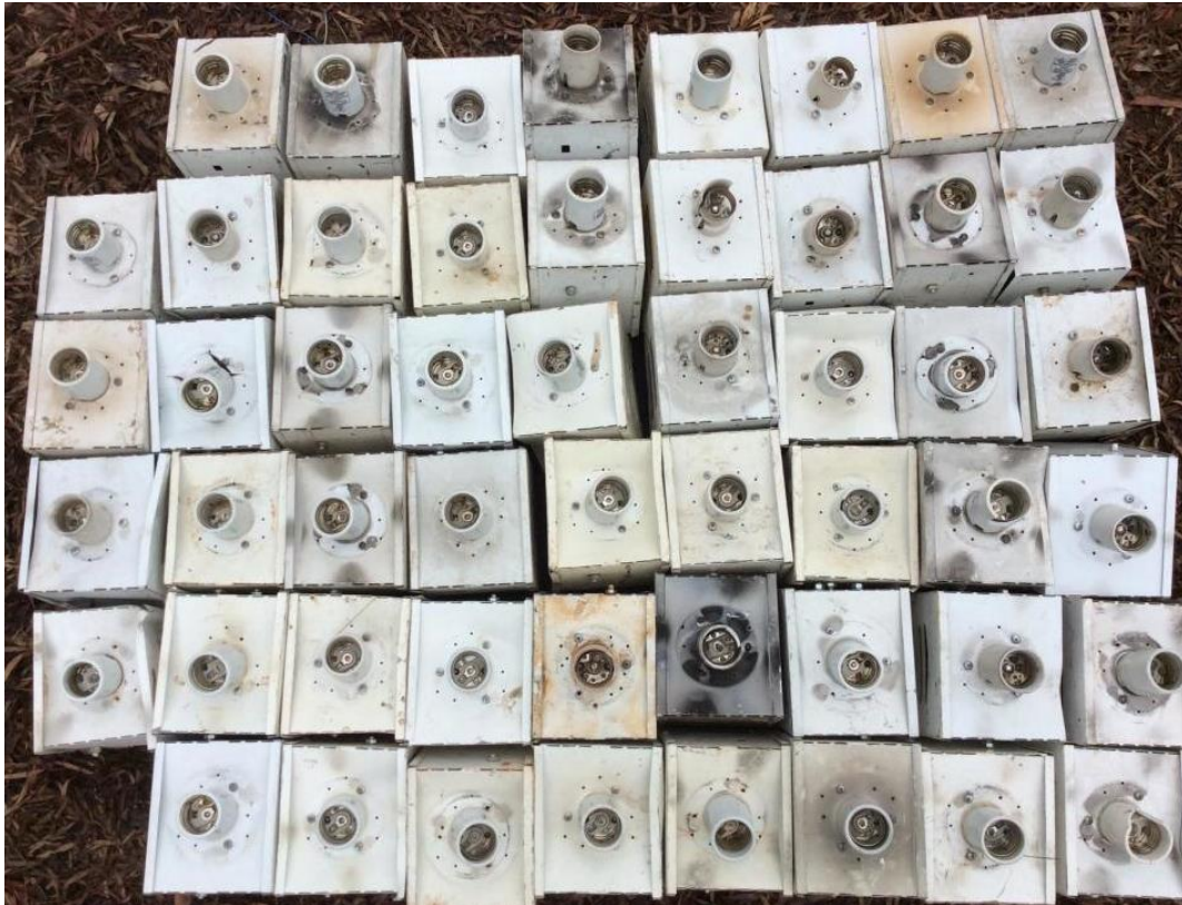
Figure 10: Example of a geo-tagged photograph of the removed ballast boxes of high-bay lamps lined up in a row with the lamp holders facing up and in focus.
