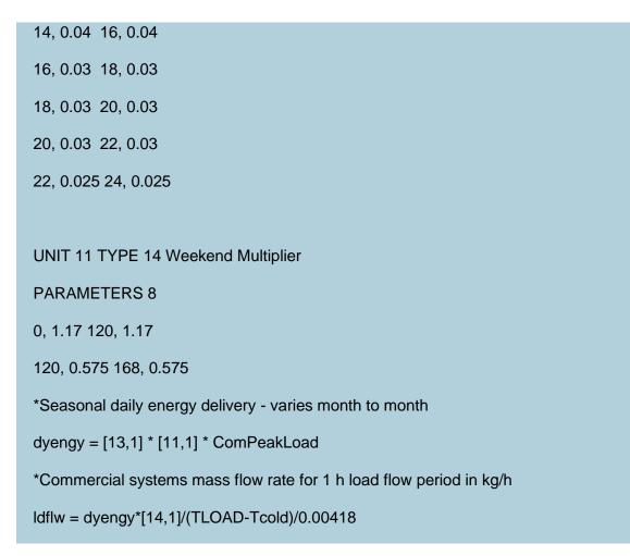
Note: [13,1] is the seasonal load pattern, TLOAD = 45°C, and Tcold is the cold water temperature, as defined in AS/NZS 4234. ComPeakLoad is the peak daily winter load as defined by the TRNSYS modeler (in the deck file), such that the system meets the performance requirements (see item 3. below).
