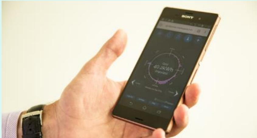
In 2015, an Australian company, Reposit Power, developed a control module (named the GridCredits system) for battery storage systems that automatically manages the energy supply and demand of a household with distributed generation (via solar PV and a battery system in this case-study). The control module automatically determines an optimal balance of supply and demand to increase financial return for the householder, and creating network benefits by smoothing the output from solar PV.
