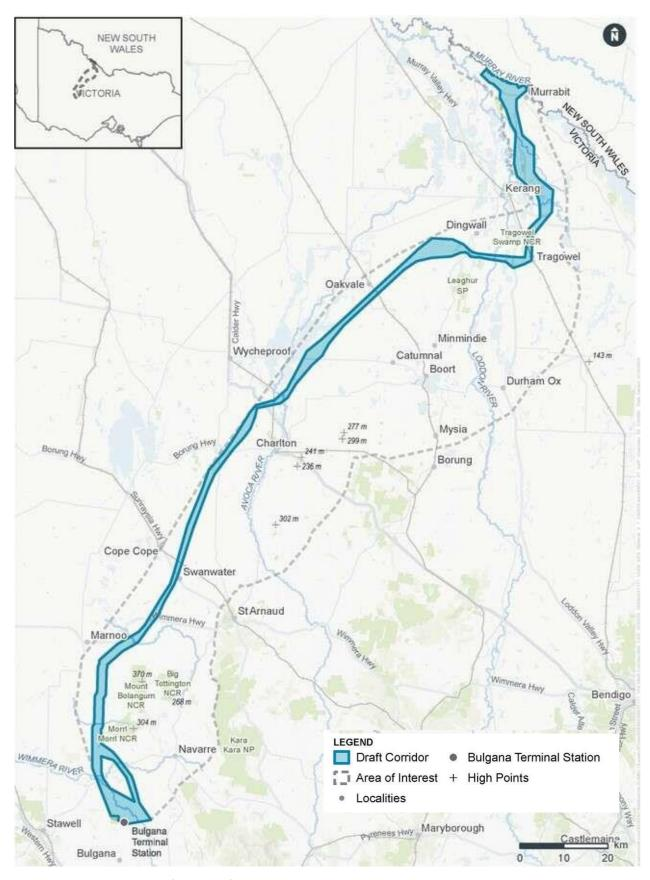
The map above shows the draft corridor for VNI West, which is approximately 2 km wide. A 70-120 metre wide transmission easement will be identified within the corridor in the next phase of the project.
