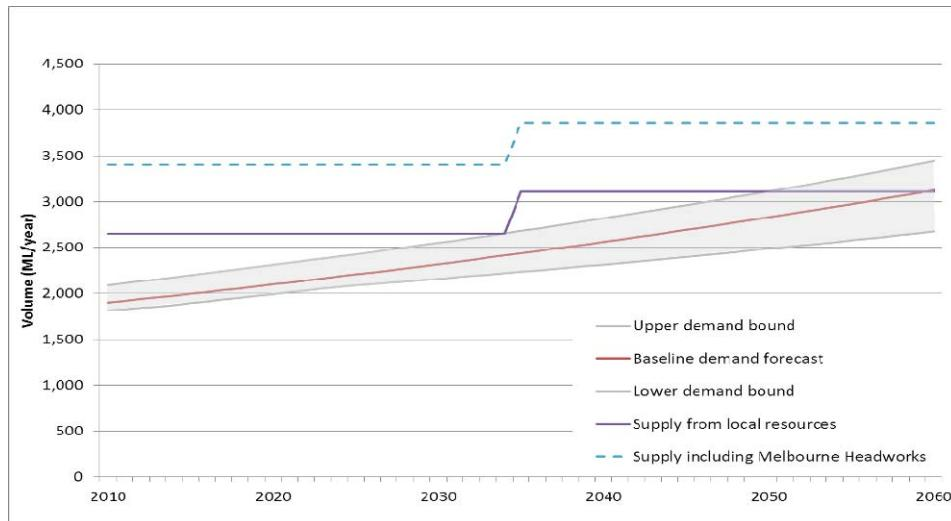
As can be seen by the chart, the forecasted supply from sources such as Candowie Reservoir, Bass River, Corinella Aquifer and the Metropolitan Water system will service the community until 2060, with our increased reservoir capacity, and a small increase in water sourced from Bass River (in year 2035).
